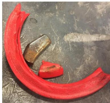
Fig 10: Pump Valve Seal and Steel Guide
