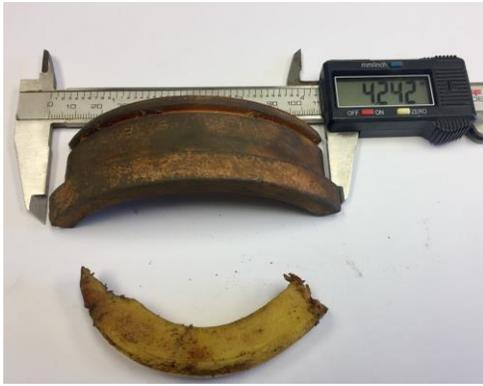
Fig 6: Weco Segment with Pump Seat
