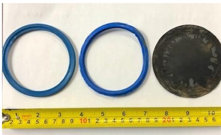
Fig 12: 3" Seal Debris
