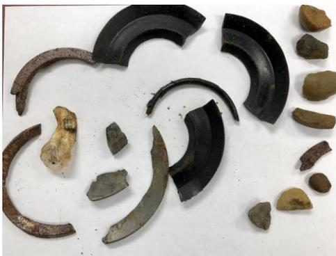
Fig 9: Metallic & Elastomer Valve Seal with Rocks
