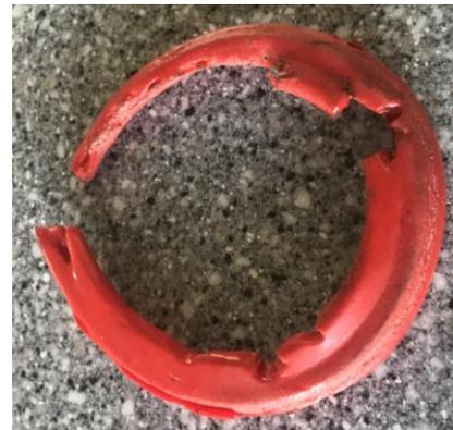
Fig 5: Pump Valve Seal (4.25")
